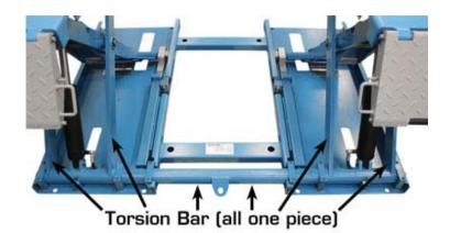
This pictures shows a lift that is not level due to poor weight placement. This caused a bind in the Passenger Side lock mechanism. The result is the Driver Side lowered and the Passenger Side stayed up. This caused the Torsion Bar to distort.
