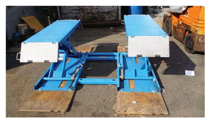
You can see that even with the lift in the fully lowered position, the Passenger Side runway is still a few inches higher than the driver side runway.
