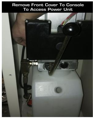
The Lowering Speed Control Valve is located directly behind the Hydraulic connection to the Power Unit. Turn Clockwise to slow the descent and Counter-Clockwise to accelerate the descent. Be sure to test the speed without weight and that you always secure anything placed on the lift according to manufacturer's specifications.
