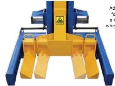
Adjustable arm forks support a wide array of wheel assemblies.
