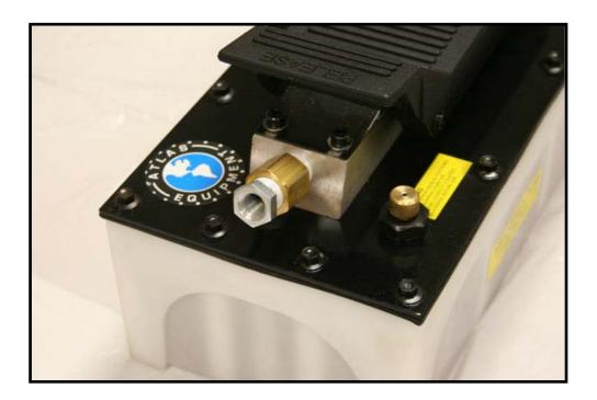
4) The Atlas Hi-Rise lift comes with a hydraulic hose already attached to the hydraulic cylinder. In order to attach the other end of the hose to the HTTLA5100 air/hydraulic pump you will need to remove the "Pointed" fitting installed on the end of the hose. Once the "Pointed" fitting is removed screw the end of the hydraulic line into the open end of the reducer you already installed in the HTTLA5100 pump.
