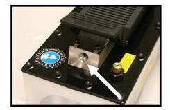
3) Thread the calibrated fitting/reducer into the hydraulic pump and tighten securely.
