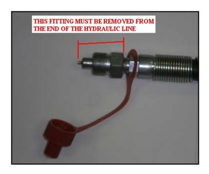
5) Check all fitting connections. Make sure they are tight enough to prevent leaks. Do not over tighten the fittings. The pump is now ready for use with the Atlas Hi-Rise 1500 Lift. The pump will connect to the lift as shown below:
