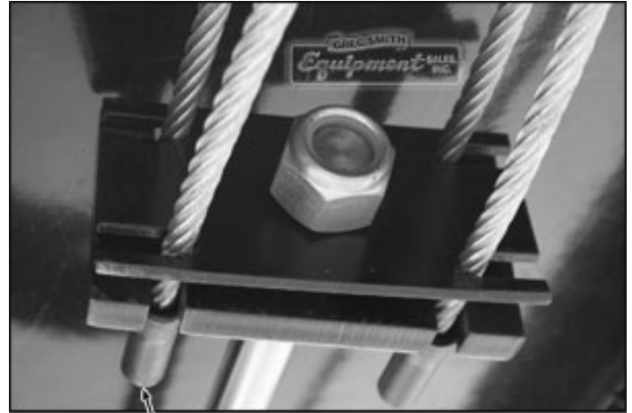
Crimped end of lift cable
