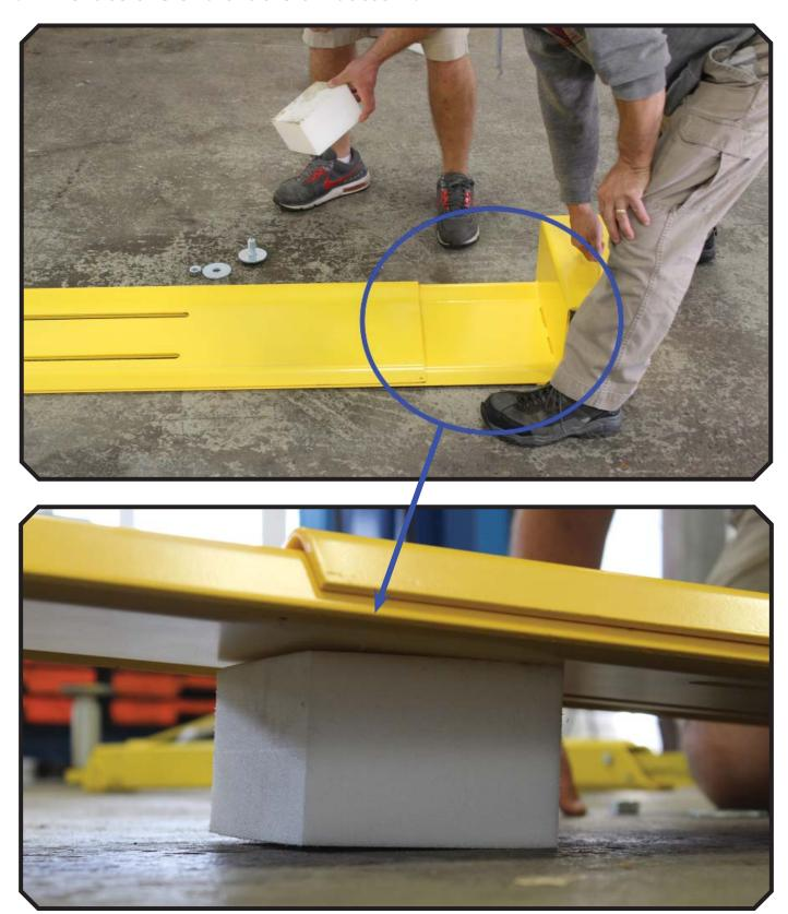
8. Install the hardware. But do not tighten with a wrench until you have the Lawn Mower Adapters on the lift arms.
