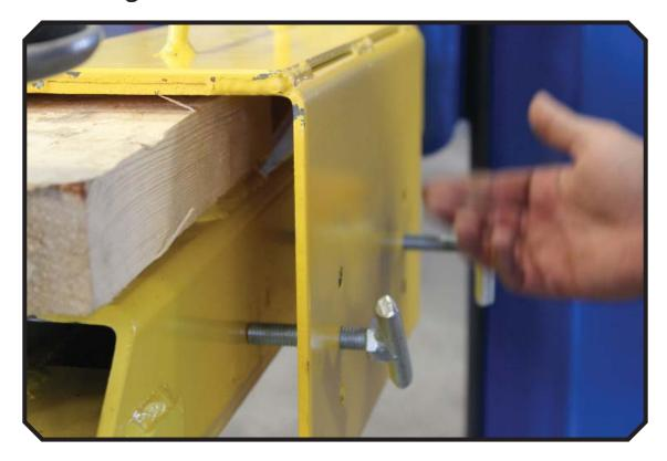
15. If the Lawn Mower Adapter sits flat on the arm without the need for a shim, screw the "T" bolts underneath the arm.
