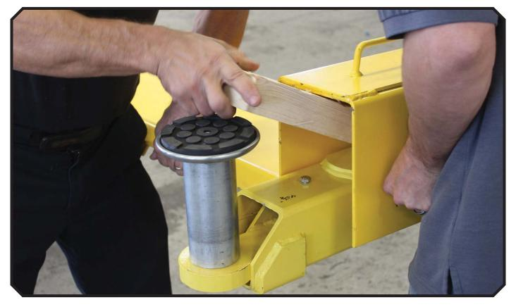
13. Use a level to ensure the Lawn Mower Adapter is resting flat on the lift arms.
