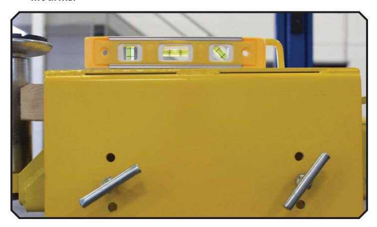
14. Once level, tighten the "T" bolts into the lift arm.
