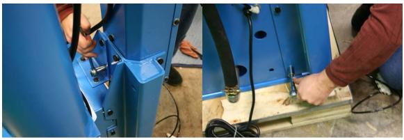
**STEP 13:** Remove the pivot bolt from the bracket shown below. Insert the Pressing Arm into the bracket and reinstall the pivot bolt.
