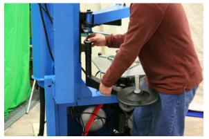
**STEP 16:** Remove the small socket head screw from the Pressing Arm. Slide the Pressing Block onto the Arm and reinstall the screw.
