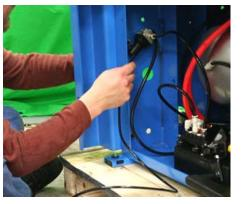
**STEP 18:** Locate the main air line inside the tire changer chassis (this line connects to the front of the lubricator/regulator and enters through the right side of the chassis). Cut this line and install the 5 way fitting on the air line as shown. The line from the Assist Arm will also reconnect to this fitting.
