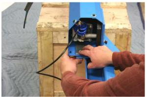
**STEP 7:** Install the Support Bracket with the 2 remaining bolts (removed in Step 3) as shown.
