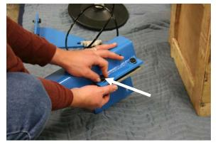
**STEP 5:** Position the Column Bracket against the Column as shown. Install the mounting bolts removed in Step 3. Do not install the bolts into the locations indicated by the arrows, set these aside for now. Do not tighten the bolts completely. This will allow you to adjust the bracket's position later.
