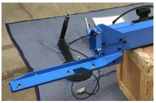
**STEP 9:** Remove the attaching bolts from the Column brackets.
