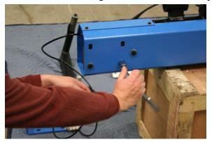
**STEP 4:** Remove the support block from the Column Bracket.
