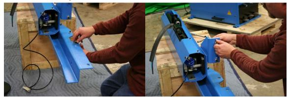
**STEP 10:** Remove the side cover from the Tire Changer.
