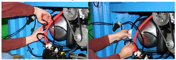
**STEP 19:** Tighten all mounting bolts. Connect the machine to a compressed air supply and check for air leaks. Install the side cover. Your LH Assist Arm is now ready to use.
