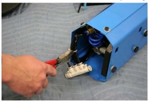
**STEP 3:** Remove the mounting bolts from the bottom portion of the Column.
