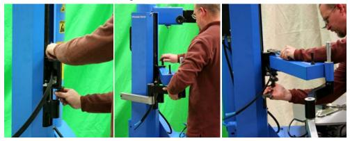
**STEP 14:** Route the air lines though the middle of the Pressing Arm. Attach the lines as shown.
