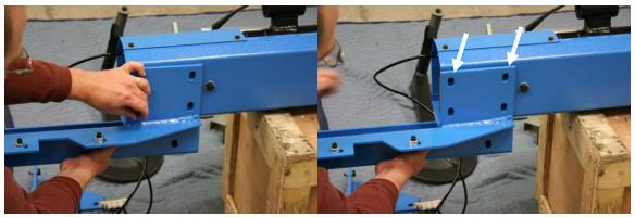
**STEP 6:** Set the support block inside the Column as shown. Install the bolts removed in Step 4 though the Bracket, Column, and into the support block.
