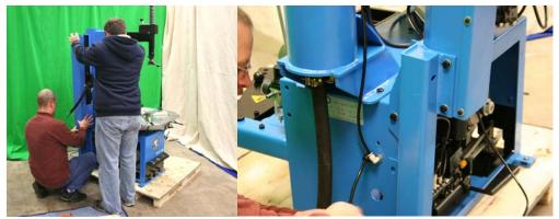
**STEP 12:** Install the attaching bolts removed in Step 9. Install the top bolts first, and then install the bolts on the rear. Do not tighten the bolts fully until all are installed.
