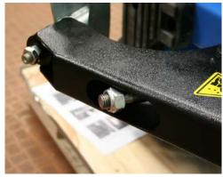
**STEP 8:** Use the locking handle to lock the hex shaft into place. Remove the bolt and cap from the top of the hex shaft. Set the cap and bolt nearby.
