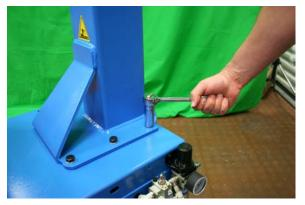
**STEP 4:** Remove the bead breaker pivot bolt and nut. Set them nearby. You will need them in a later step. Install the round rubber pad onto the bead breaker shaft (arrow). Position the bead breaker arm onto the chassis as shown.
