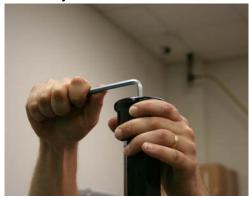
**STEP 9:** Slide the coil spring over the hex shaft. Push the spring downward and install the cap and bolt (removed in step 8) to hold the spring into place.
