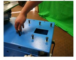
**STEP 3:** With an able bodied helper, carefully lift and position the main column as shown. Install the six bolts removed in step 2. Tighten the bolts securely with a socket wrench.
