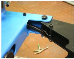
**STEP 6:** Align the holes in the chassis and bead breaker arm. Install the pivot bolt and nut.
