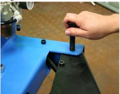
**STEP 7:** Guide the bead breaker shaft through the pivot pin (on the breaker arm). Install the locknut using a socket wrench and extension. If an extension is not available to you, you may pull the breaker shaft outward to access the shaft and nut with a wrench.
