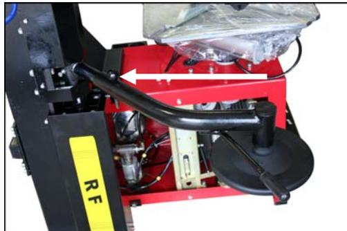
**STEP 28:** Congratulations! Your Tire Changer Assist Arm is complete. Remember to check all bolts and screws for tightness. Connect air and electrical service to the machine. Set the air regulator between 100 and 116psi.and check thoroughly for air leaks. Test each function and control on the machine as described in the owner's manual **BEFORE** attempting to change tires. **THE TIRE MACHINE SHOULD BE OFF OF THE SKID BEFORE OPERATING.**
