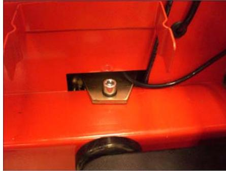
**STEP 22:** Find the two lines from **STEP 18** inside the machine. Press the line marked “C” into the upper right fitting (located at the left rear, inside the machine, next to the regulator) as viewed from inside the Chassis. Press the line marked “D” into the lower right fitting. These connections will match the lines installed on the outside of the machine in **STEP 11**.
