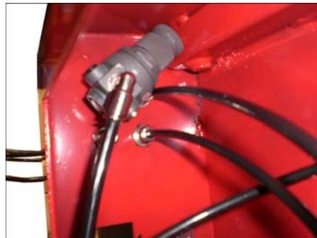
**STEP 23:** Remove the stop bracket and Allen screw from the end of the Roller Arm (left photo). Slide the Roller arm through the mounting bracket as shown in the right photo. Reinstall the stop bracket and Allen screw.
