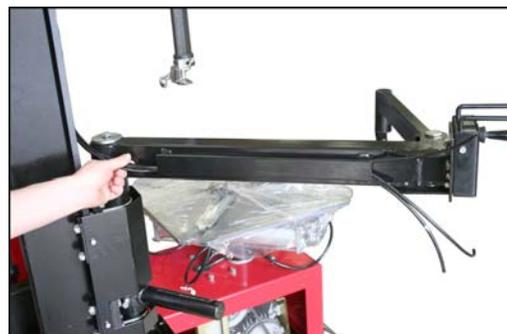
**STEP 17:** Press each of the five marked lines into the matching numbered port on the Assist Arm control box.
