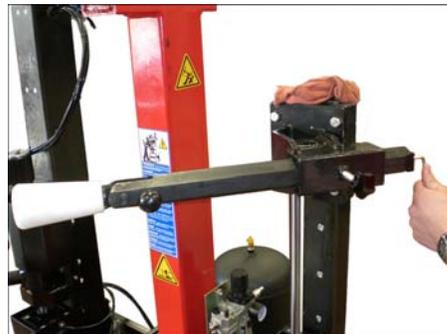
**STEP 24:** Remove the two nuts from the Right Disk Arm (top left photo). If desired, apply a light coat of grease to the Right Disk Arm shaft before installing. Insert the shaft on the arm into the mounting bracket from the bottom up (top right photo). The hole is located to the left of the Roller Arm. Reinstall the two nuts onto the shaft. Tighten the nuts against each other, allowing enough free play for the arm to swing freely.
