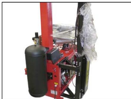
**STEP 12:** Locate the two air fitting holes in the rear of the Main Chassis (arrows). Remove the two bulkhead fittings from the Hardware Kit (bottom photo). Remove one nut from each fitting and install them as shown in the right photo. Reinstall the nuts onto the fittings to hold them firmly in place.
