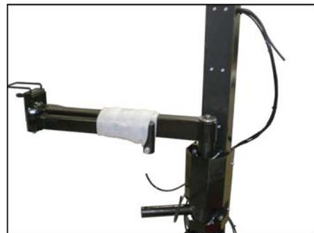
**STEP 16:** Locate the loose air lines coming out near the top of the Assist Arm Column. Route the five longest lines (labeled 1, 2, 3, E, and F) through the square tube on the back of the Pressing Arm as shown above.
