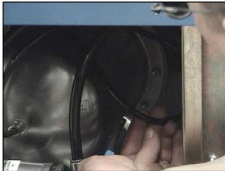
**STEP 9:** Locate the Hose Tee Assembly included with the Assist Arm. Connect the cut ends of the air supply line into the Hose Tee as shown. Press the hoses into the press lock fittings completely make certain they are tight.
