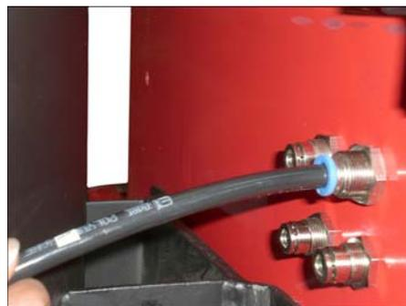
**STEP 14:** Press the hose marked “B” into the lower right fitting (top left photo). Press the hose marked “C” into the upper left fitting (top right photo). Press the hose marked “D” into the lower left fitting (bottom photo). Make sure all of the hoses are pushed fully into each fitting. This will ensure a good seal.
