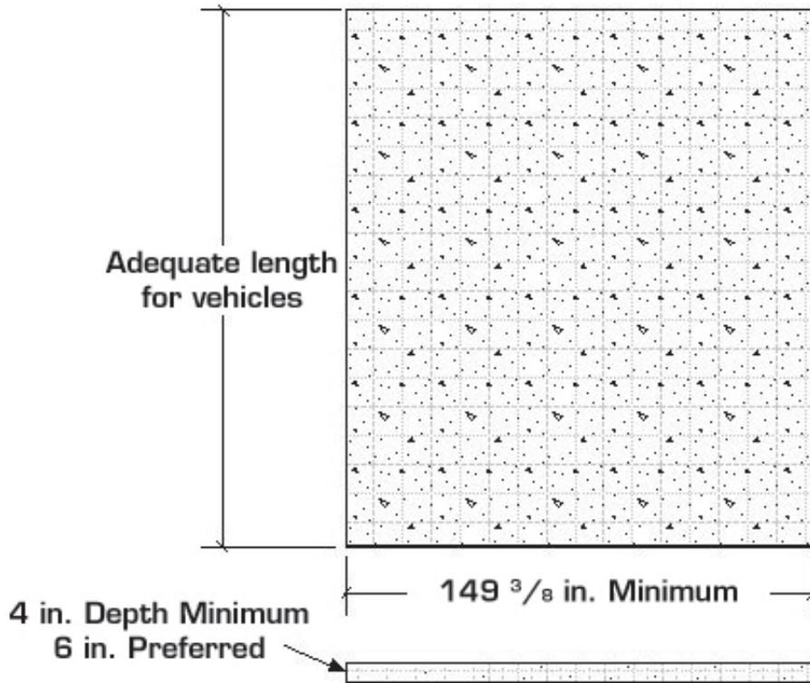
1. Concrete shall have compression strength of at least 3,000 PSI and a minimum thickness of 4" in order to achieve a minimum anchor embedment of 3 1/4". NOTE: When using the standard supplied 3/4" x 5 1/2 long anchors; if the top of the anchor exceeds 2 1/4" above the floor grade, you DO NOT have enough embedment.
