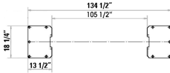
8. Use the existing holes in column base plate as a guide for drilling the 3/4" diameter holes into the concrete. Drill the anchor holes only for ONE column, installing anchors as you go. You will install anchors in second column after the cables, hoses, and floorplate are installed.
