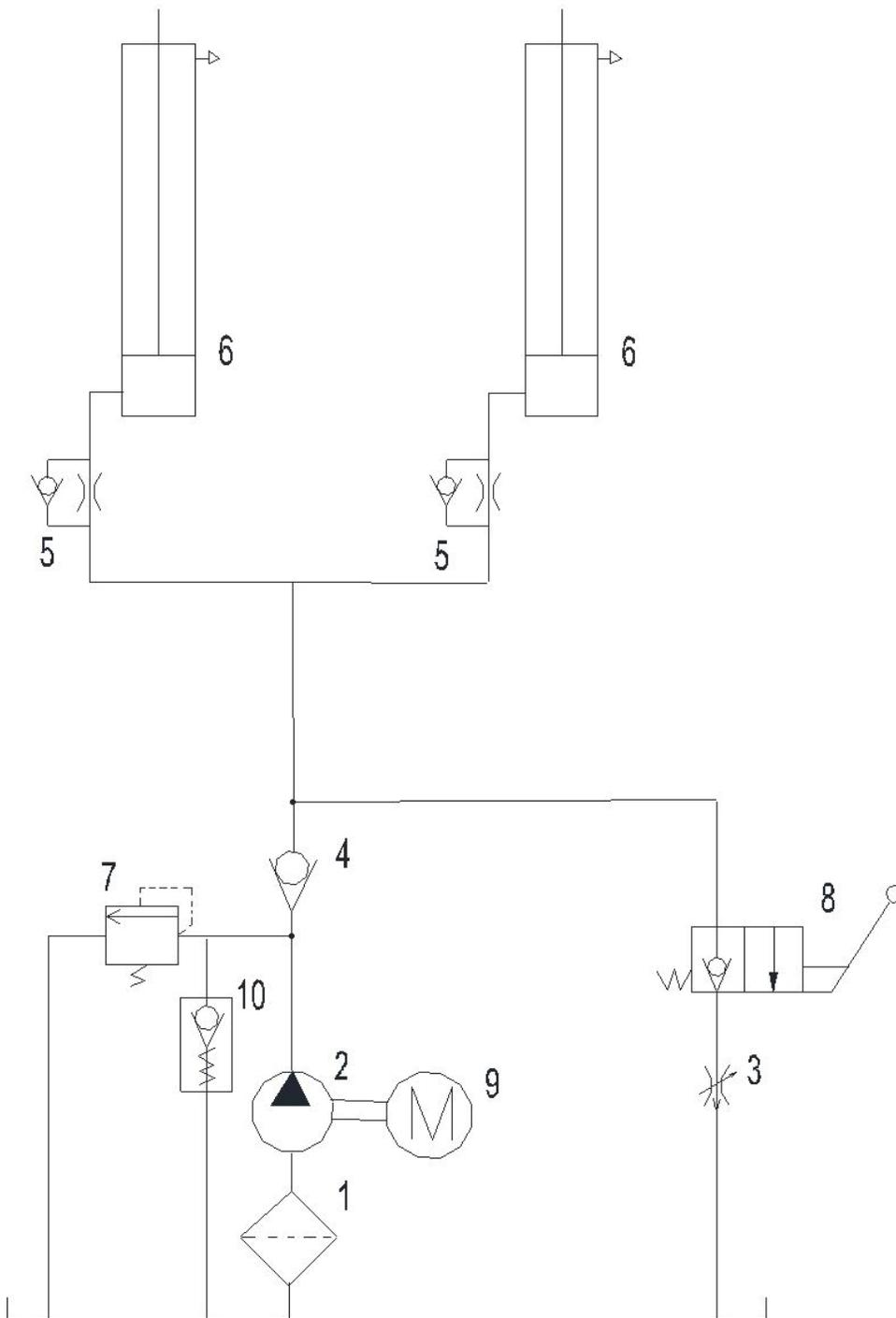
Figure 5 - Hydraulic Plan
