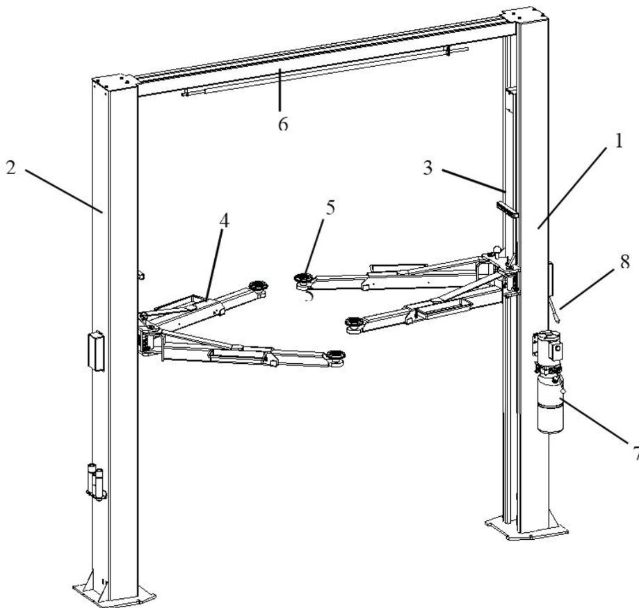
Raising motion is carried out by pushing the lifting button on a power unit (7) which delivers the hydraulic fluid to cylinders inside the columns to act on the chain system to raise the lift. Lowering the vehicle by pushing down the lowering handle on the power unit while holding down the safety lock handle (8).
