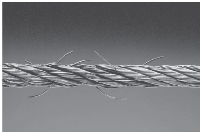
Cable with Broken Wires
