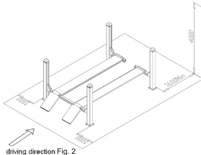
2. **FLOOR REQUIREMENTS:** The lift should be installed on a 3000 PSI concrete with little gradients. Thickness of concrete  $\geq 6$  inch (150 mm). The leveling of whole area  $\leq 3/8$  inch (10 mm). Or, every column shall be located on a concrete block with size at least 24\*24 inch (600\*600 mm), thickness  $\geq 8$  inch (200mm)
