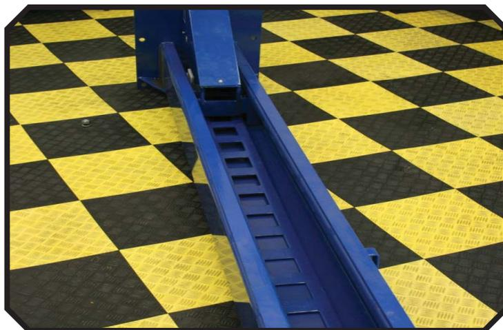
5. Insert the **long locking ladders** through the cross beams. Using the bolt supplied at the bottom of the column, attach the long lock ladders. **Do not tighten the bolt.** (Refer back to Installing Rear Cross Beam steps 3 & 5.
