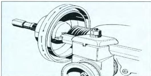
*Figure 13 - Positioning the boring bar*
