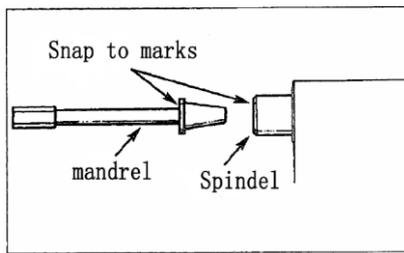
Figure 3-Align witness marks during arbor installation
