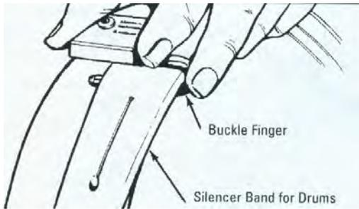
*Figure 12-Attach silencer band*
