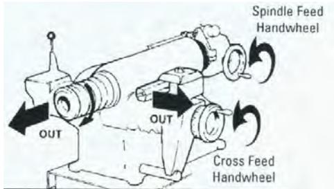
Figure 10-Counterclockwise rotation of handwheels
