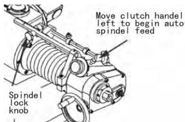
Figure 19 – Spindle auto feed
