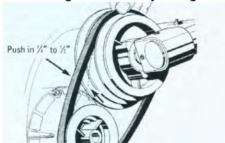
Figure 8-Press the belt in and tighten adjusting nut
