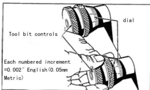
Figure 26 – Tool bit controls
