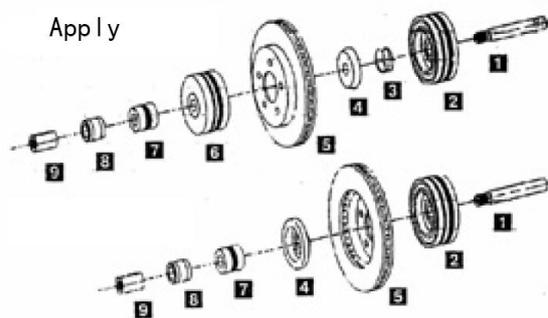
1-1" Arbor 2-Flange Plate 3-Spring 4-Centering Cone 5-disc 6- Flange Plate 7-Spacer 8-Self-Aligning Spacer 9-Arbor Nut
