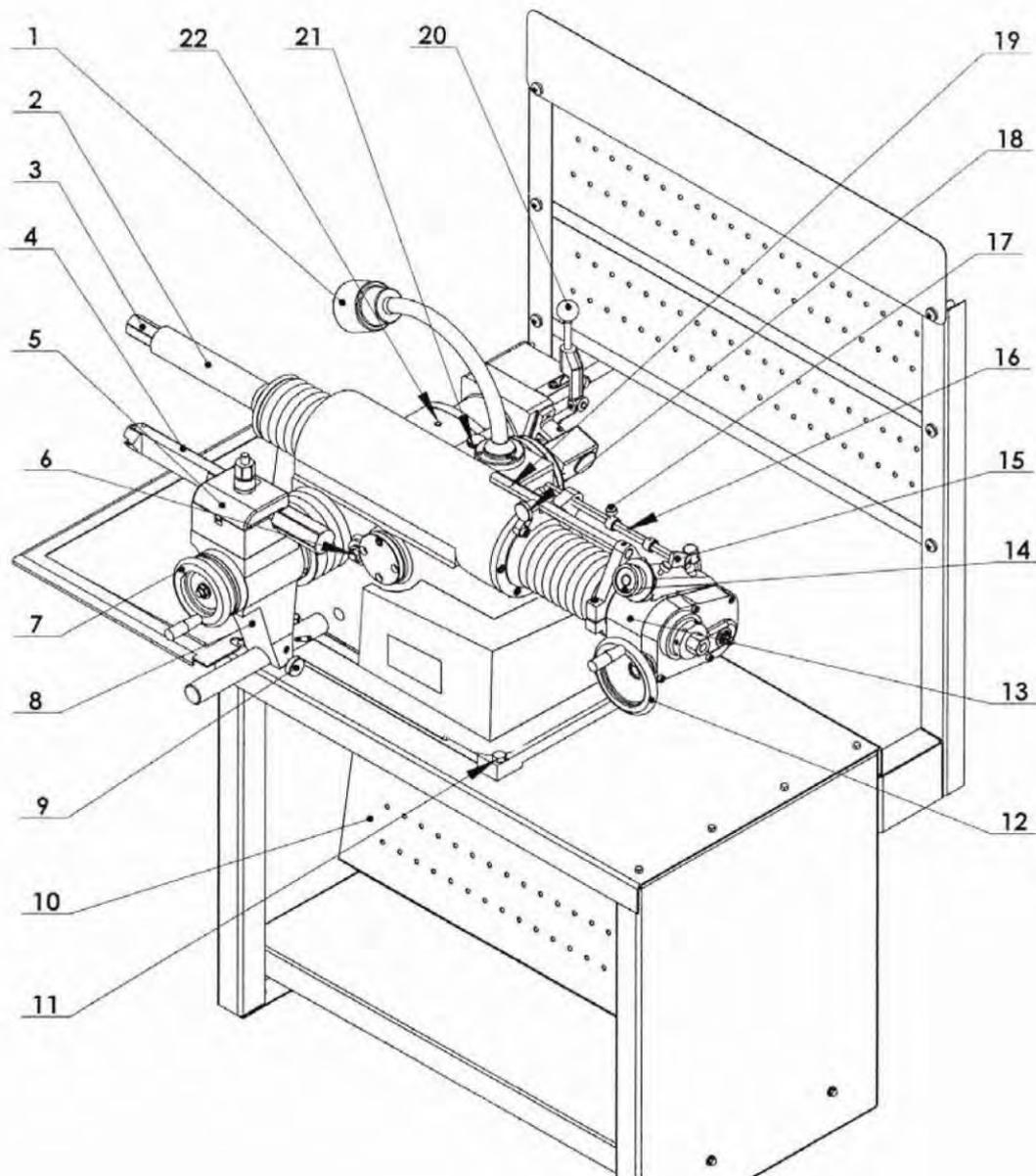
1-Work Light 2-Spindle 3-Spindle Nut 4-Boring Bar 5-Boring Bar Clamp 6-Oil Plug 7-Cross Feed Handwheel 8-Cross frame 9-Cross Feed Lock 10-Bottom Plate 11-Bolt 12-Spindle Feed Handwheel 13- Spindle Feed Gearbox 14- Spindle Feed Dial 15- Spindle Feed Clutch Lever 16- Spindle Travel Control rod 17- Control rod Lock 18- Spindle Lock 19- Spindle rod 20- Cross Feed Adjusting Lever 21-Oil Dipstick 22-Grease Fitting
