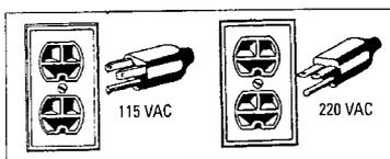
Figure 1-Power Cord Plug and Receptacle Types
