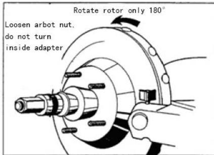
Figure 28 – Rotate rotor 180°
