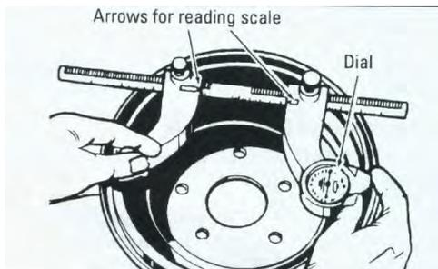
Figure 11-Measure drum diameter
