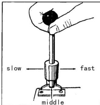
Figure 31 – Engage automatic cross feed
