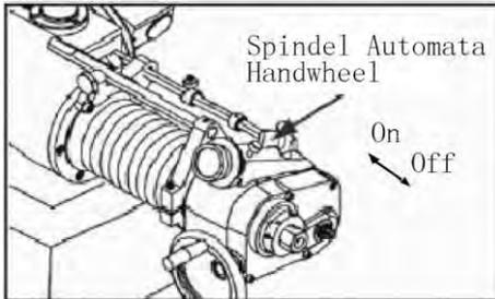
Figure 5- Spindle Feed Clutch
