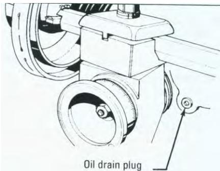
*Figure 33 – Drain plug location*
