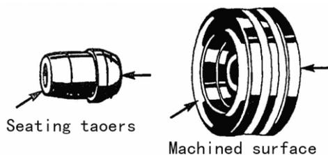
Figure 4-Use care to avoid damaging mating surfaces
