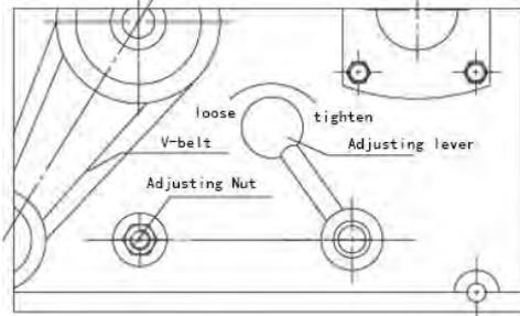
Figure 7- Loosen nut and Engage lever
