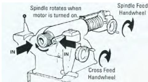
Figure 9-Clockwise rotation of handwheel
