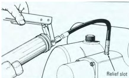
*Figure 34 – Cross feed grease fitting*
