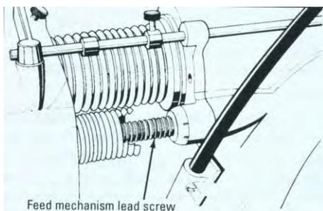
*Figure 35 – Feed screw pole*
