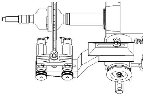
Figure 24 – Center the twin cutter
