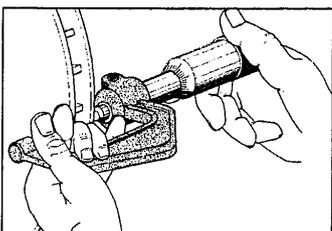
Figure 20 – Measure rotor thickness
