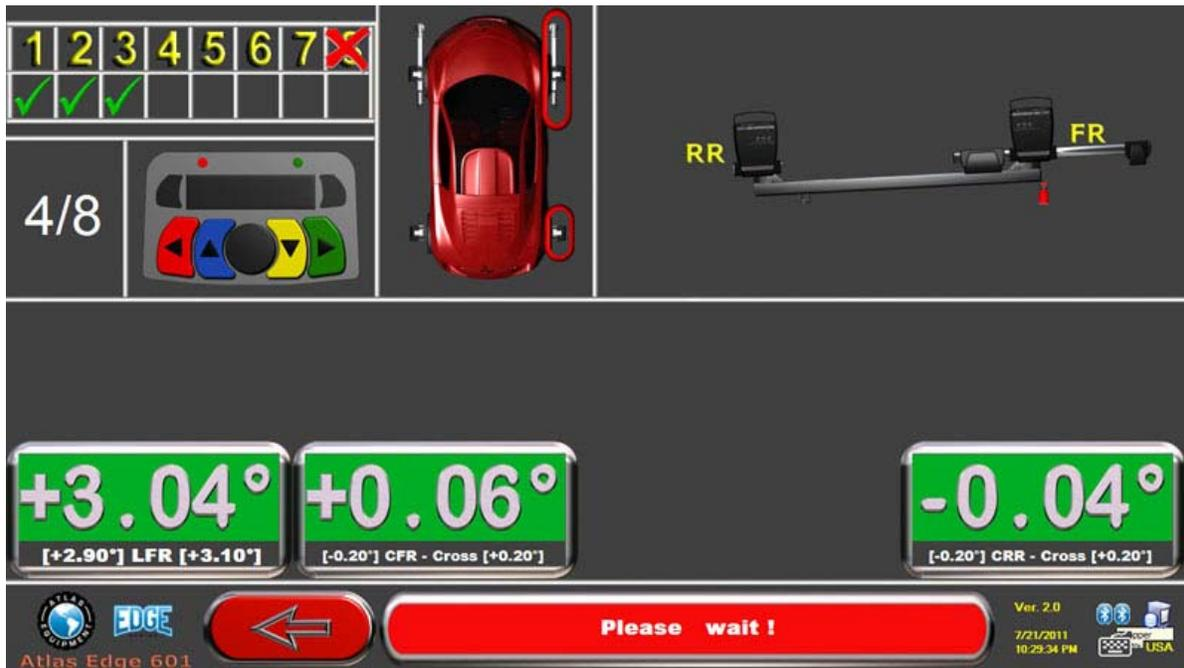
Press "F5" on the keyboard or the middle Black Sensor Button to proceed and finish calibrating the FR and RR sensors.
