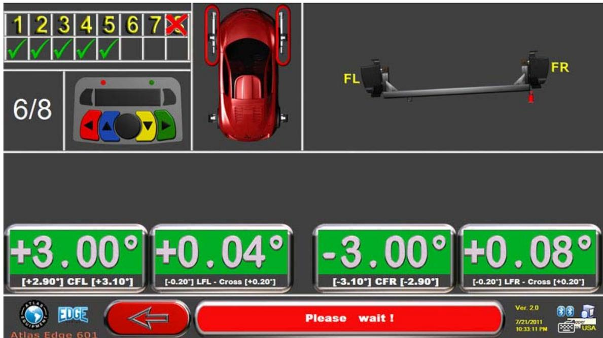
Press "F5" on the keyboard or the middle Black Sensor Button to proceed and finish calibrating the FL and FR sensors.
