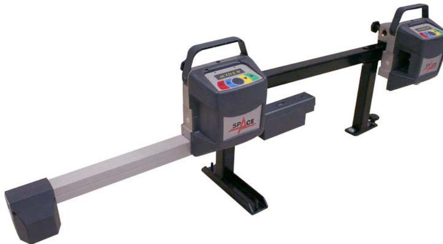
**(Figure A)** To calibrate the Left Front and Left Rear Sensors configure the Sensors on the calibration bars as shown above. The Sensors are labeled. The **RIGHT** sticker on the back of the sensor head will be labeled according to Sensor position. **(F.R., R.R., F.L., R.L.)**
