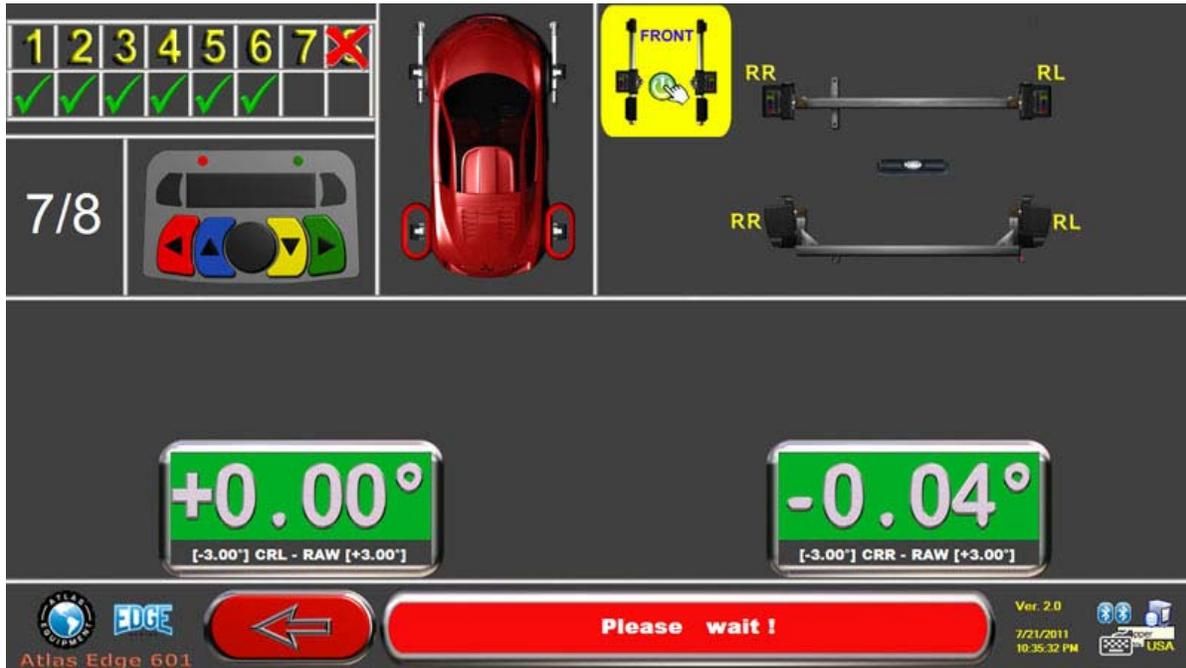
Press "F5" on the keyboard or the middle Black Sensor Button to proceed and the RR and RL Sensors will calibrate.
