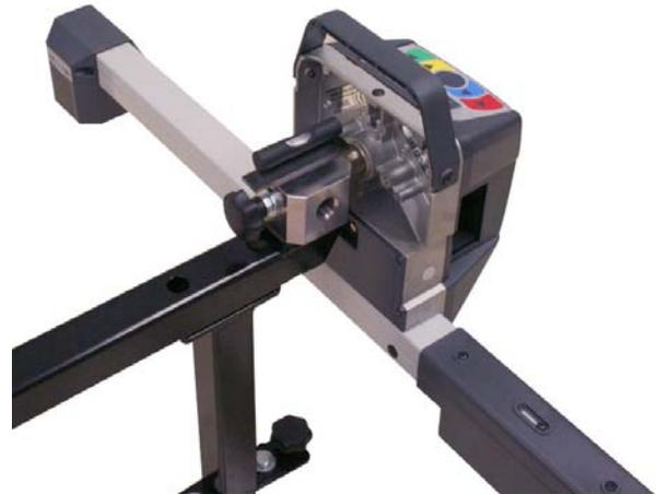
Before you proceed, ensure that your alignment calibration bar is level using the provided precision leveling tool. Check the steel block on the **knob adjuster side** of the calibration bar and ensure that they are level.
