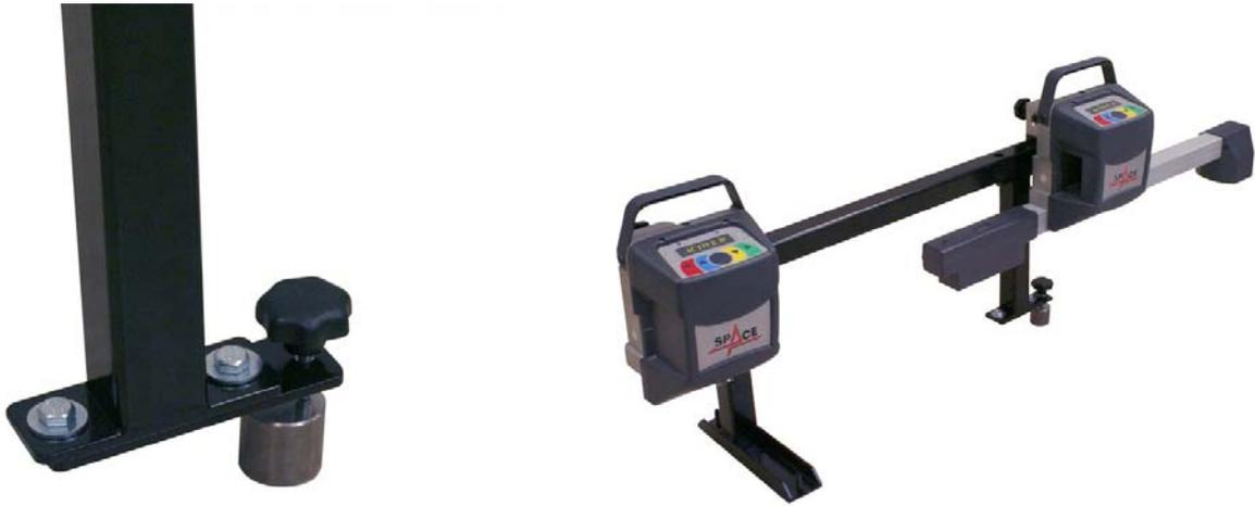
Raise the Rear of the Calibration Bar by 3 degrees using the Provided Steel Slug.
