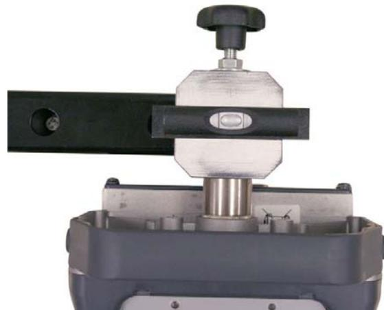
Ensure the Front Sensor bar and the calibration bar is level.
