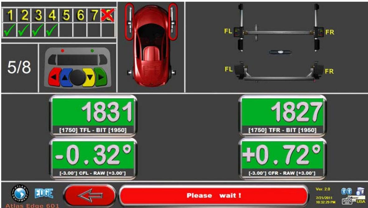
Press "F5" on the keyboard or the middle Black Sensor Button to proceed and the FL and FR Sensors will begin calibration.
