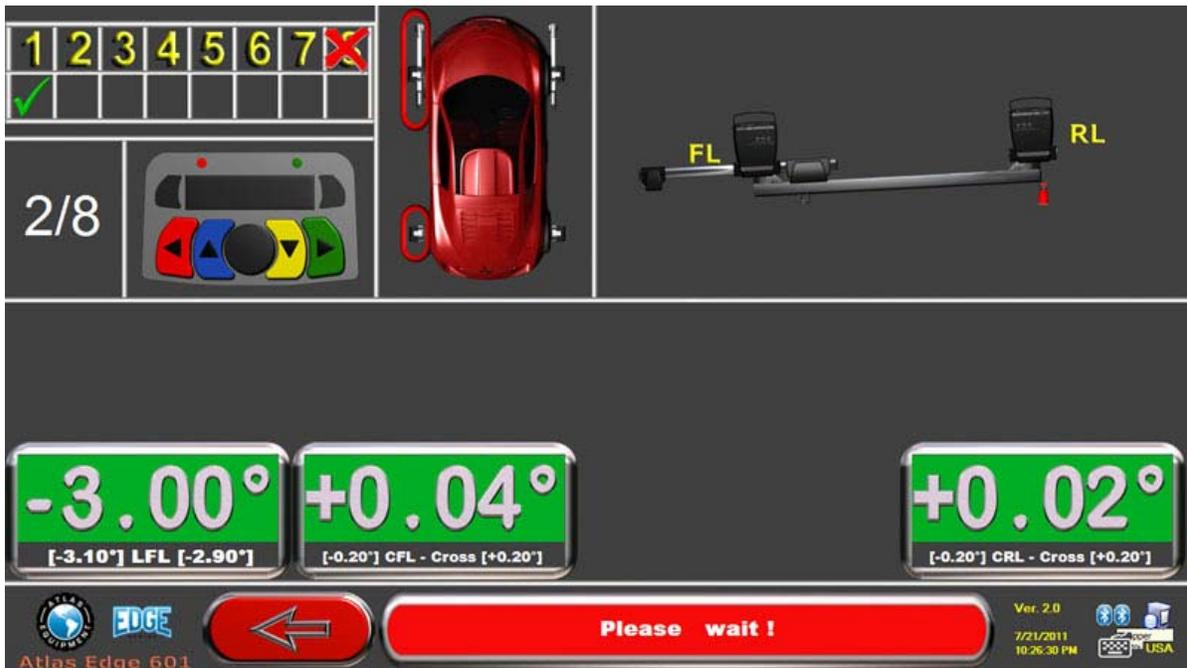
Press "F5" on the keyboard or the middle Black Sensor Button to proceed and to finish calibrating the FL and RL sensors.
