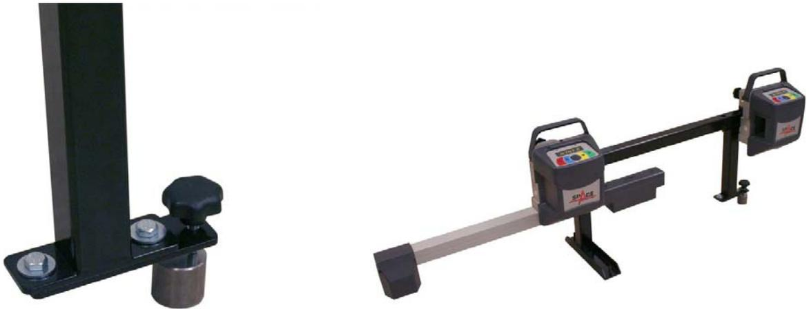
Raise the Rear of the Calibration Bar by 3 degrees using the Provided Steel Slug.
