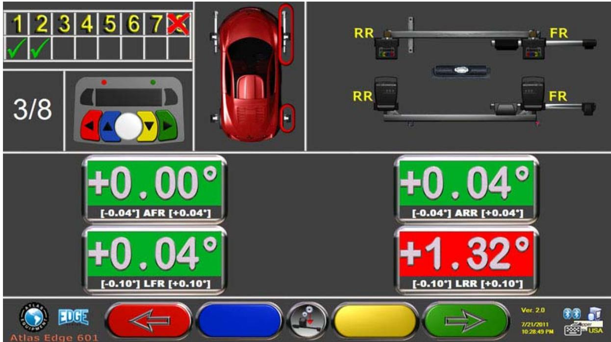
(Figure A) To calibrate the Right Front and Right Rear Sensors configure the Sensors on the calibration bars as shown below. The Sensors are labeled. The **RIGHT** sticker on the back of the sensor head will be labeled according to Sensor position. (**F.R.**, **R.R.**, **F.L.**, **R.L.**)
