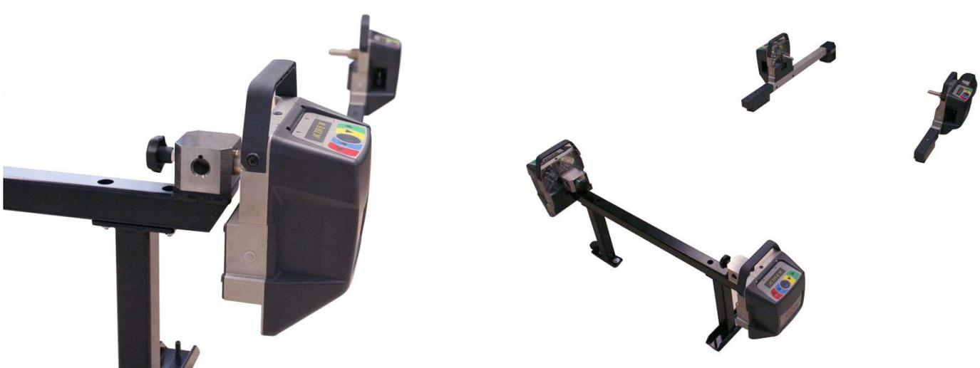
Position the Front Sensors somewhere nearby. The Rear Sensor Cameras must have line of sight with the Front Sensor Cameras in order to establish a signal.
