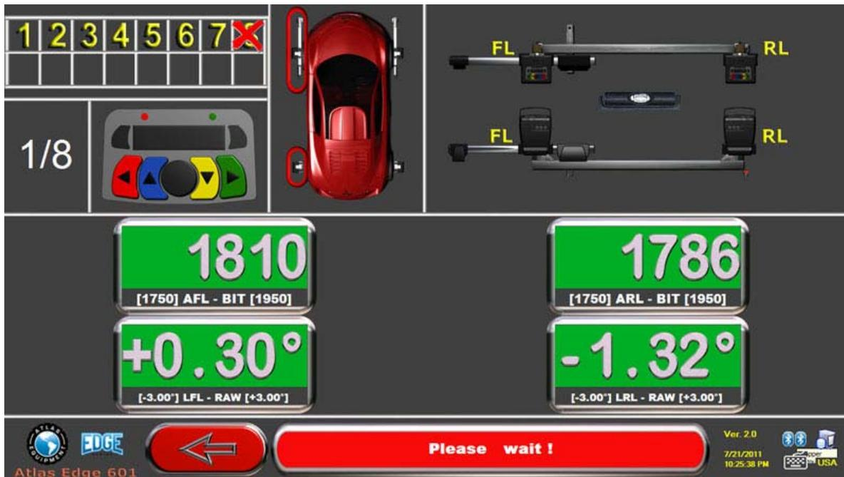
Press "F5" on the keyboard or the middle Black Sensor Button to proceed and the FL and RL Sensors will begin calibration.
