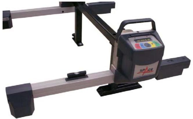
Tighten the sensors into the sockets using the provided fastening bolts.
