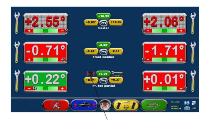
To unfreeze the caster values- Move the red R to the caster position using the center key on the head or the F5 on the keyboard.
