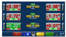
Adjust toe on left wheel to preferred target.
