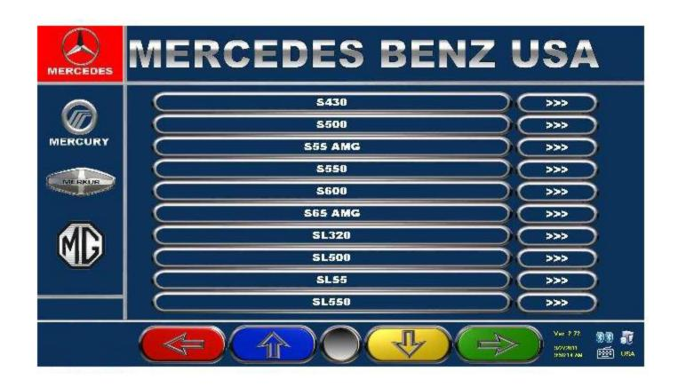
Choose vehicle manufacturer from the column on left by scrolling or by entering the first letters of the manufacturer name. Chosen manufacturer will be highlighted in red box. Select the green key and select the model in the same manner.
