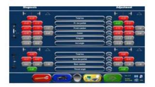
Final print screen indicates diagnosis, adjustment, and target data values for both axles. Select red key to view additional measurement screen or yellow key to print/store.
