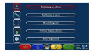
When viewing additional measurements use the **blue** and **yellow** keys to scroll up or down. Select **green** to print/store.
