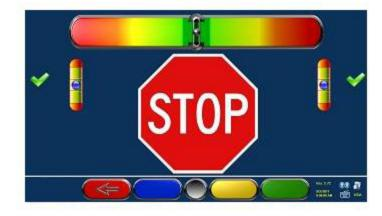
Level the front sensor heads until vials on screen are centered and indicate OK with green check marks. Then steer the front wheels in the direction indicated by the arrow on screen until the centering ball icon is in the green area in the center of the bar graph. The STOP sign appears then hold the position steady.
