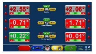
After adjustments are completed press blue key before lowering vehicle. Lower and select center black key on sensor head to confirm that vehicle has been lowered.
