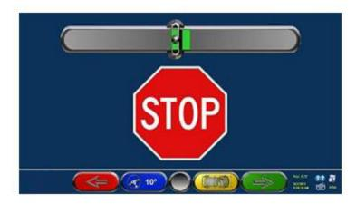
Turn wheels to left until ball and carriage icon is in the green area on the slide. Hold position steady until screen changes. Now turn wheel to the right and repeat. When screen changes steer back to the center until the red stop sign appears.
