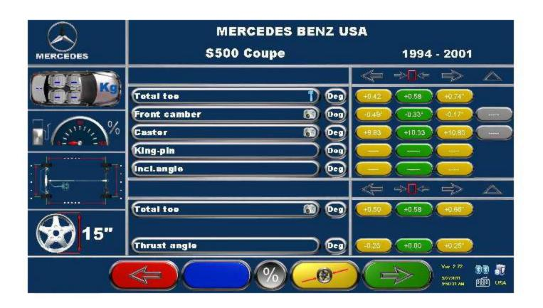
If the correct vehicle has been selected advance by selecting the green key. If not select the red key to reselect the vehicle. If you are measuring toe in millimeters you may change rim size with the yellow key. Otherwise select the green key to advance to the next step.
