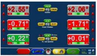
Red UP arrows are now visible on each side of screen. Make caster/camber adjustments with straight ahead steering position. Do not re-level sensor heads.
