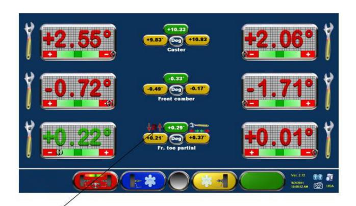
Adjustment of Partial Toes- With steering wheel lock installed and steering wheel in the straight position set left and right toe to the same value and on preferred specification.
