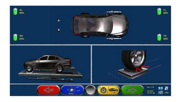
Runout Compensation Skipped – If using Atlas Non-Runout Fast Clamps select the green key to move forward. Runout Compensation Method- Select the yellow key to choose between raised and rolling runout methods. Front Axle Measurement Using Only Two Sensor Heads- Select the blue key to measure toe and camber on the front axle with only two sensor heads installed.
