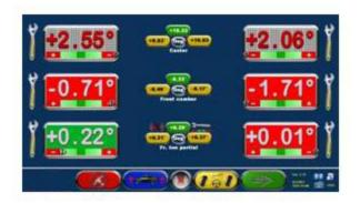
After adjustment of front toe select green key to move forward to the final printout screen.
