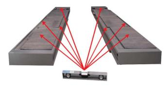
to working position (ramps at different heights) but to do this, it is has to start from a known condition: **LIFT LEVELED AT THE GROUND POSITION!!**
