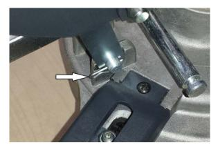
Insert the clips to lock the pin.
