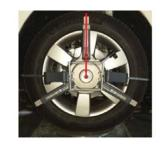
In the rear part of the Target, there is a label which identifies the working position.
