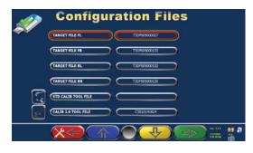
The Target files are located in the memory stick that came with the PC. Check on the memory key, in the "TARGET" folder, the files stored have the same name of the target mounted on Clamps. Connect the USB to the PC.
