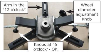
Connect the quick locking device on the clamp
