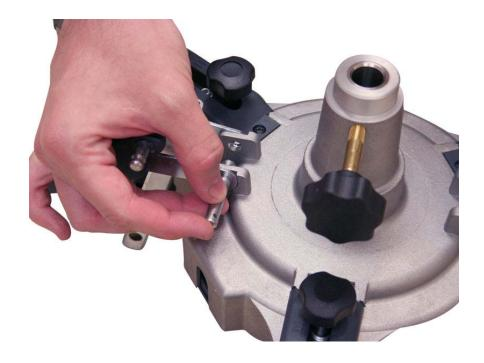
Locate one of the Arm Support Pins (Part 4) and fit it through the holes of the Clamp Handles (Part 6) and Fast Clamp Base (Part 1) as shown and lock the Support Pin into place using 2 of the Pin Locking Clips (Part 3)
