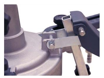
Both of the Fast Clamp Handles (Part 6) should now be securely fastened to the Fast Clamp Base. (Part 1)
