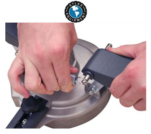
Attach the first Arm Spring (Part 2) to the notched pins located at the top of the clamp handles as shown. (Part 6)
