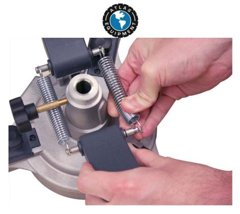
Attach the second Arm Spring (Part 2) to the other side of the notched pins located at the top of the clamp handles as shown. (Part 6)
