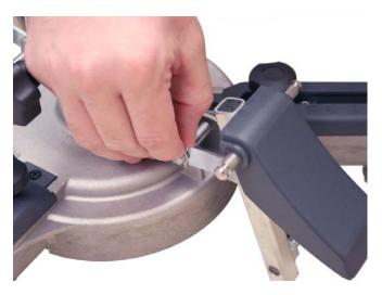
Use the second Arm Support Pin (Part 4) and fit it through the holes of the Clamp Handles (Part 6) and Fast Clamp Base (Part 1) on the opposite side of the clamp as shown and lock the Support Pin into place using 2 of the Pin Locking Clips (Part 3)
