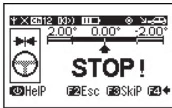
**Fig 45 Put Straight Steering Wheel**
