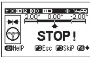
**Fig 45 Put Straight Steering Wheel**
