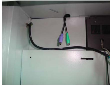
Put computer display on the cabinet top cover. Insert the power wire and data wire of the display into the oblong hole on the top of the back cabinet and pull them out to insert into the power and data sockets on the display. Insert the other end of the data wire into the display interface on the host computer. Insert the power wire into the power socket at the top of the inside cabinet. See Fig. 25 and 27.
