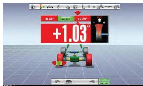
**Fig. 78 Single Wheel Adjustment**
