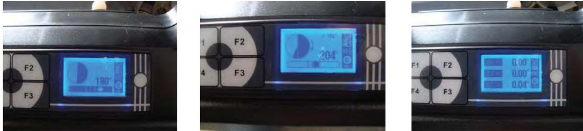
For lift-up compensation, it should be done one wheel by one wheel without strict compensation sequence.
