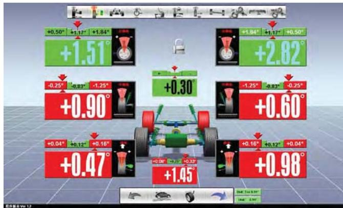
Fig. 79 Front Wheel Adjustment
