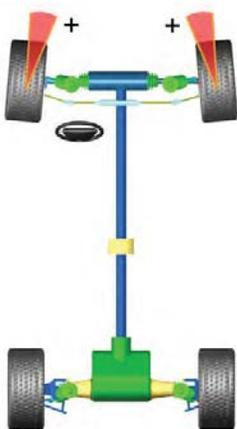
Toe-in is the angle drawn by a line drawn through the plane of one wheel referenced to the longitudinal axis of vehicle. Toe-in is measured in positive or negative degrees. Positive toe-in is when the horizontal line intersects in front of the vehicle. Negative toe-in is when the horizontal line intersects behind the wheel. Total toe-in is the total of the front toe measurements, i.e. the angle formed by two horizontal lines
