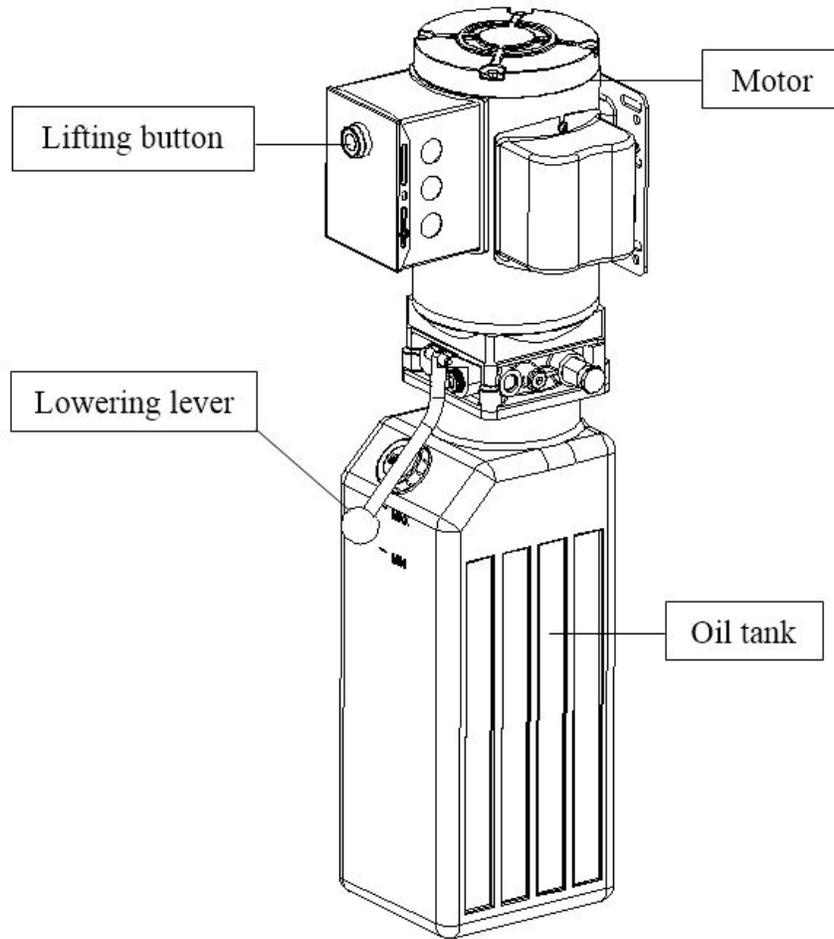
Figure 3 – Hydraulic Power Unit
