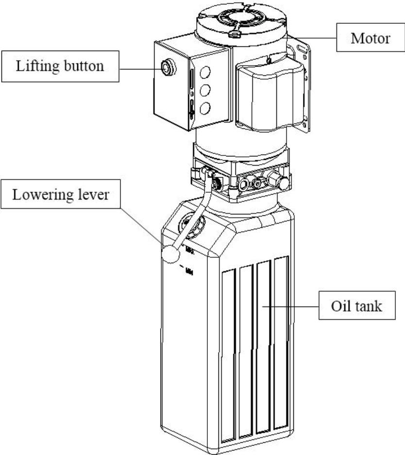
Figure 3 – Hydraulic Power Unit
