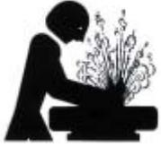
If a higher inflating pressure is required remove the wheel from turntable and continue the inflating procedure inside a special protection cage (commercially available).
