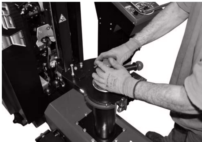
Install the calibration jig on clamping chuck
