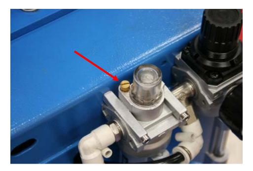
The Brass Screw (arrow) is the Flow Adjustment for the Lubricator. Turning this screw will change the flow rate of oil dispensed by the Lubricator. Turning the screw counter-clockwise (left) will increase the oil flow. Turning the screw clockwise (right) will reduce the oil flow.
