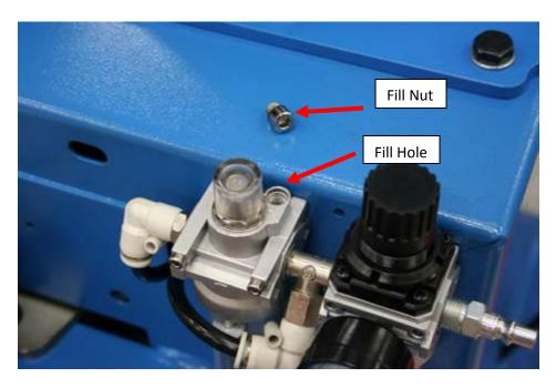
Locate the Silver Fill Nut (see above). After removing the Fill Nut you will be able to fill the reservoir with Air Tool Oil.
