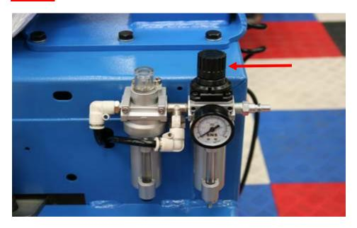
Located the Pressure Adjusting Knob (arrow). Lift the knob slightly to unlock the knob. Turning the knob clockwise (right) will increase the air pressure level. Turning the knob counter-clockwise (left) will reduce the air pressure level. Set the Pressure Gauge to between 110 and 120psi. The FRL
