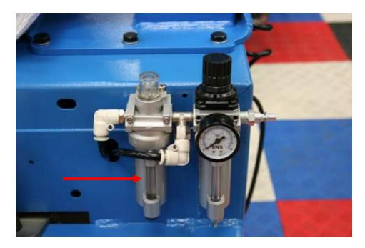
Fill the reservoir until you can see the oil level at or, near, the top of the sight glass (arrow). Replace the fill nut. The adjustment of the flow rate will be adjusted after the Air Pressure Gauge is adjusted.
