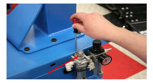
Use a flat blade screwdriver to adjust the flow by turning the screw in  $\frac{1}{2}$  to  $\frac{1}{2}$  turn increments. To correctly adjust the flow rate, watch the sight glass on top of the Lubricator (arrow). Operate the bead breaker through its full travel several times. The correct flow rate adjustment will cause a drop or mist of oil to appear in the sight glass every 2-3 times that the bead breaker is operated.
