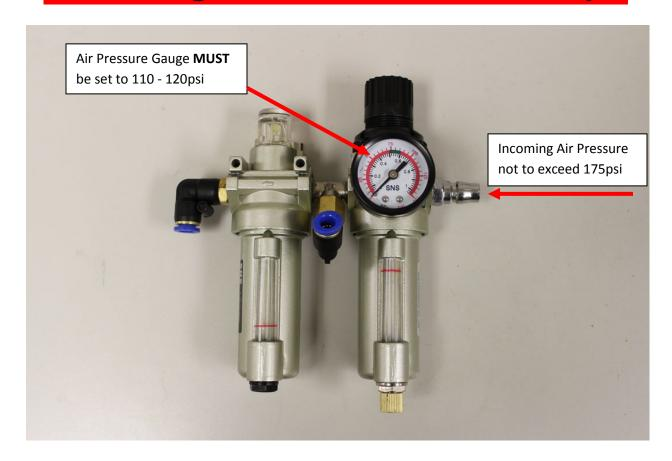
This guide will explain how to adjust the air pressure and the flow rate of the oiler. Failure to follow these guidelines will void the Warranty.
