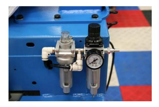
The Filter Regulator Lubricator is located at the rear of the Tire Changer on the Right Hand side when facing the front of the machine. Before any air is connected to the machine it is the owner's responsibility to fill the Lubricator with Air Tool Oil. Once air is connected to the FRL the air pressure
