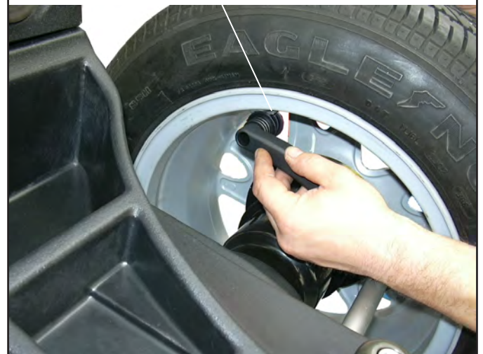
Fit weight on the position where pliers touches the wheel
