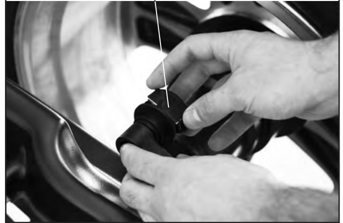
Fig. 38 Fit the adhesive weight in the pliers of the gauge rod
