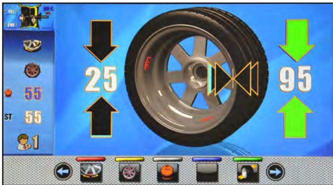
Fig. 38 Fit the adhesive weight in the pliers of the gauge rod
