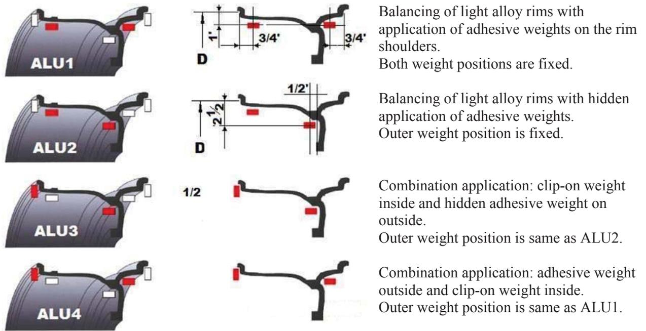
Balancing of light alloy rims with application of adhesive weights on the rim shoulders. Both weight positions are fixed.
