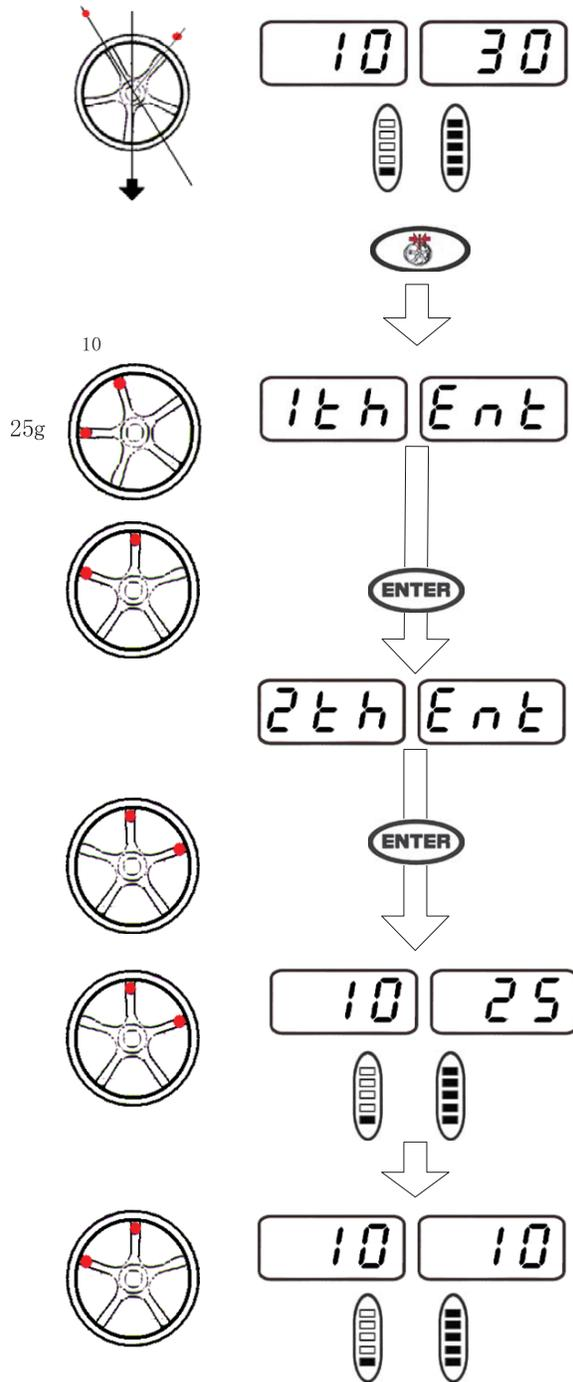
At ALU☆ mode, the unbalanced amount of the outer side of the rim shown on the digital readouts is 30g.
