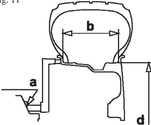
**A:** The distance, measured from the machine to the inner side of the rim
