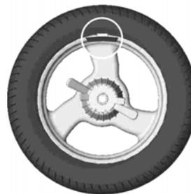
Figure 6.6 - The weight is set in the "12 o'clock" position
