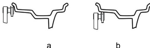
Figure 5.3 - Placing the gauge arm during the first measurement
