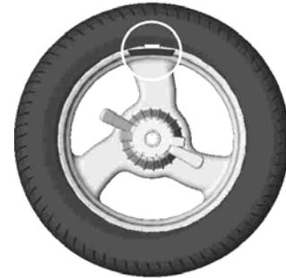
a - display image while clip-on weight setting    b - weight is set in the "12 o'clock" position
