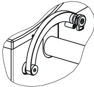
Figure 4.2 – Initial position of the gauge arm
