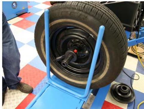
**STEP 6:** Install the car extension on the measuring rod.
