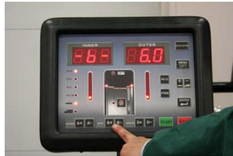
“D” (diameter of the wheel in inches; (refer to marking on tire))
