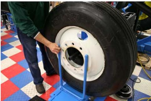
**STEP 4:** Place the cone on the shaft..
