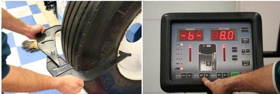
“D” (diameter of the wheel in inches; (refer to marking on tire))
