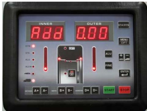
**STEP 16:** Give the wheel a push to get it spinning, lower the hood, and spin the wheel. Giving the wheel a “push start” reduces the strain on the motor.
