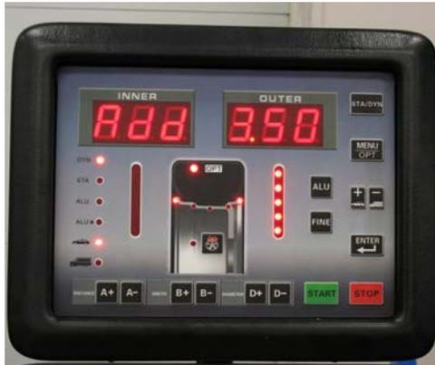
**STEP 18:** After the cycle is finished, the screen will flash “EEP ON” then return to “000 000”. Your balancer is now calibrated. To check the calibration, rotate the wheel so that the weight is positioned at 6 o’clock. All of the weight indicators should be fully lighted as shown below.
