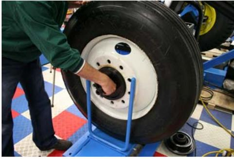
**STEP 5:** Finally, place the Heavy Duty Nut on the shaft and tighten securely.
