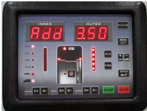
**STEP 19:** After the cycle is finished, the screen will flash “**EEP ON**” then return to “**000 000**”. Your balancer is now calibrated. To check the calibration, rotate the wheel so that the weight is positioned at 6 o’clock. All of the weight indicators should be fully lighted as shown below.
