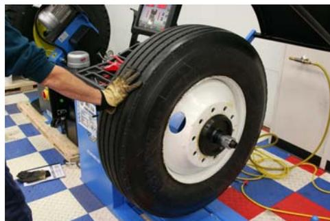
**STEP 17:** When the cycle is finished and the tire stops, the display will read “**3.50 Add**” (**100 grams**). Rotate the wheel until all the inside weight indicators are fully lighted. Apply the **3.5 ounce (100 gram)** truck calibration weight (shown below) on the inside edge of the wheel at the 12 o’ clock position. “Push start” the wheel, lower the hood, and spin the wheel.
