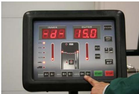
**NOTE:** The measuring rod used to determine the “A” distance is marked in centimeters. You must convert to millimeters by multiplying the measurement by 10. This is the value you must enter as the “A” measurement. See the examples below:
