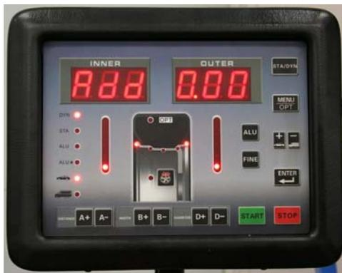
**STEP 16:** When the cycle is finished and the tire stops, the display will read “**3.50 Add**” (**100 grams**). Rotate the wheel until all the inside weight indicators are fully lighted. Apply the **3.5 ounce (100 gram)** passenger car/light truck calibration weight (shown below) on the inside edge of the wheel at the 12 o’ clock position. Lower the hood and spin the wheel.
