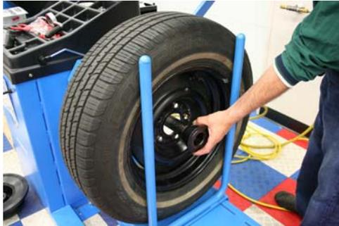
**STEP 5:** Finally, place the Quick Nut on the shaft. Tighten the Quick Nut securely, but do not over tighten.
