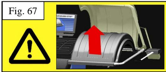
The wheel guard is raised when the machine is spinning.
