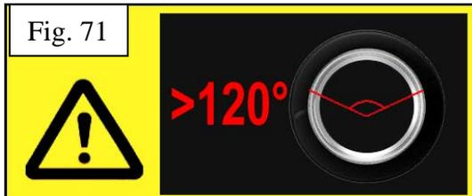
In SPLIT mode, the split angle is more than 120 degrees and cannot perform the correct split function.
