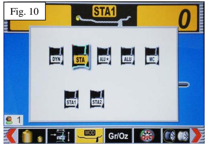
Fig. 11 – BALANCING MODE SELECTION PROCEDURE
