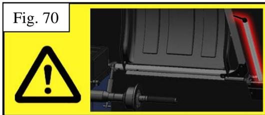
B gauge is not moved to the correct position when the gauge is needed to be set measurement. Or the B gauge is faulty.
