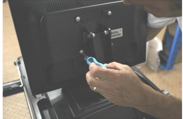
**Plug the cable in the back of the monitor and hand-tighten the thumb screws.**
