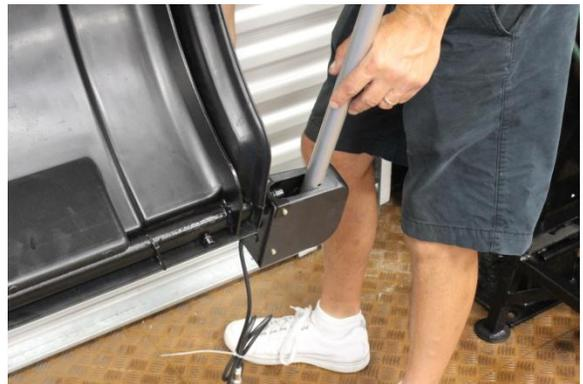
Route the "B-Gauge" cord through the nylon straps and plug it in on the side of the WB55 chassis. Tighten the nylon straps.
