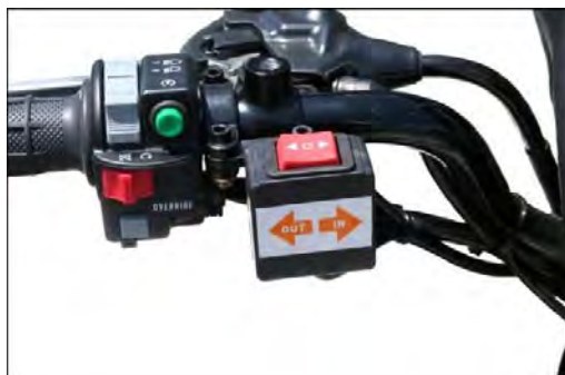
Handle Bar Switch position for IN and OUT
