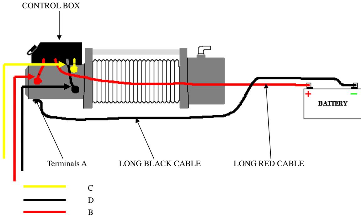
Pay close attention to proper electrical cable connection as follows (refer to Diagram1)
