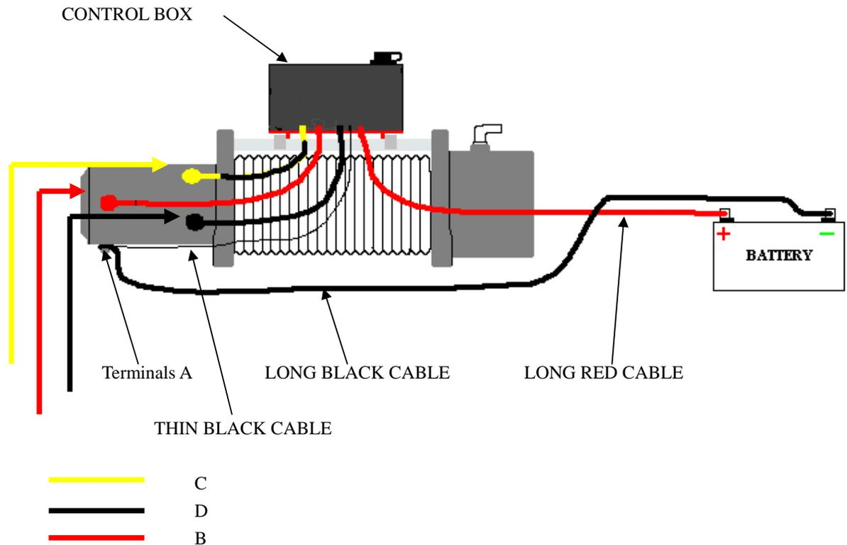
Pay close attention to proper electrical cable connection as follows (refer to Diagram1)
