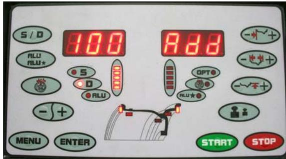
**STEP 10:** When the cycle is finished, the display will read “Add 100” (3.5 ounce). Remove the calibration weight from the inside edge of the wheel. Rotate the wheel until all the outside weight indicators are fully lighted. Apply the 100 gram (3.5 ounce) calibration weight to the outside edge of the wheel at the 12 o’ clock position. Lower the hood and spin the wheel.
