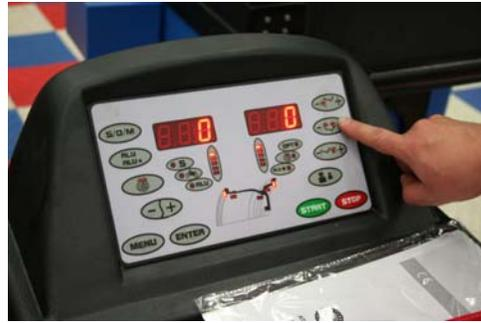
“D” (diameter of the wheel in inches; Use caliper, or refer to marking on tire)
