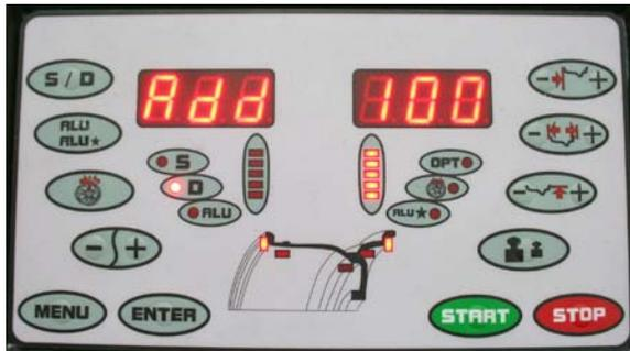
**STEP 11:** After the cycle is finished, the screen will flash “EEP ON” then return to “000 000”. Your balancer is now calibrated. To check the calibration, rotate the wheel so that the weight is positioned at 6 o’clock. All of the weight indicators should be fully lighted as shown below.
