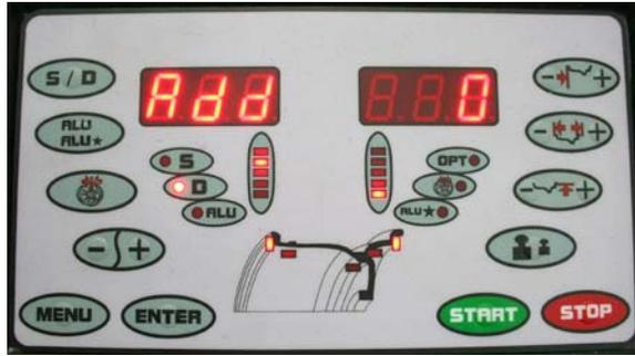
**STEP 9:** When the cycle is finished and the tire stops, the display will read “100 Add” (3.5 ounce). Rotate the wheel until all the inside weight indicators are fully lighted. Apply the 100 gram (3.5 ounce) calibration on the inside edge of the wheel at the 12 o’ clock position. Lower the hood and spin the wheel.
