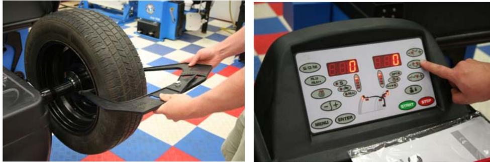
“D” (diameter of the wheel in inches; Use caliper, or refer to marking on tire)
